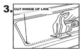
Using a saber saw, cut inside of cutout line. Trial fit sink to check proper fit.
