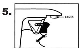
Insert the sink clips into the slots of each sink boss. Apply a bead of caulk /not included/ to the underside of the sink flange. For final fit, make sure each sink clip is pulled back as illustrated. Position the sink into the counter top opening.
