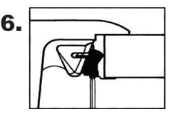
Secure the sink by pivoting the sink clips into the position illustrated and tighten screws in the front, then tighten rear and side screws.
