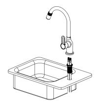
2. Put C through the base, fix C with A, as shown on the picture
